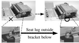
• Close the top cover by fitting its rear end lug first for ribbon replacement only or go on loading paper as in next paragraph.
